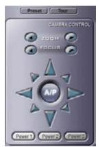
: PTZ cameras connected to DVR System can be controlled from DVR Net. The arrow buttons will move the camera in the direction of the arrow, and the ZOOM, FOCUS buttons will manipulate the camera accordingly. However, only user with permission can control the PTZ setting.
